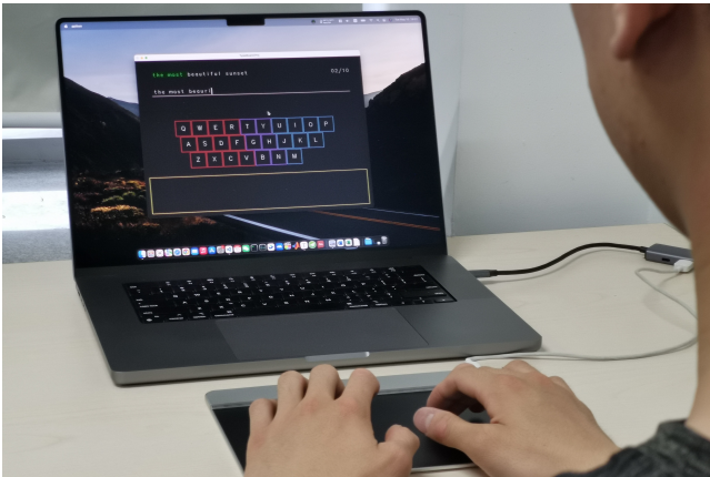
Figure 2: The apparatus used in user studies. Users type on ResType, which is implemented on a Sensel Morph touchpad. ResType is connected to a MacBookPro that shows the GUI feedback.
