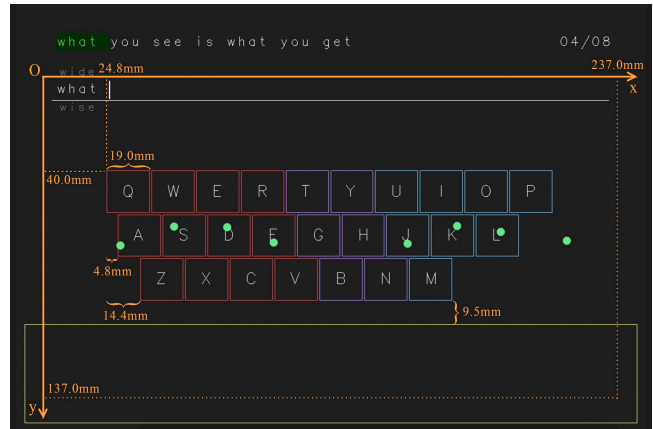
Figure 3: The keyboard layout and GUI of the final ResType. Users can only input 26 English letters and “space” in ResType. The orange annotations illustrate the keyboard range, which is linearly mapped with the touchpad sensing area and not shown to users.
