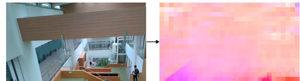
Figure 21: Illustration of VideoFlow Failure Case. At this extreme distance, human movements have become so minute that they are obscured by noise.
