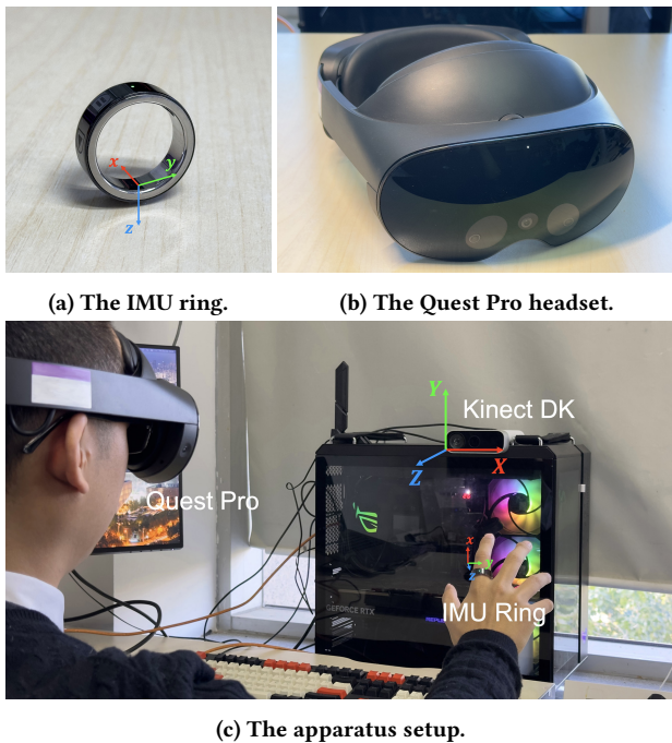
Figure 5: The apparatus setup in the user study. The user wears an IMU ring on the index finger and a Meta Quest Pro on the head. The Meta Quest Pro and the IMU ring capture the optical and inertial data respectively. We also add a Kinect DK camera to record the study process and use it as a marker of the world coordinate frame. All optical data are captured and converted to the world coordinate frame XYZ, while the IMU data are in the local coordinate frame xyz.
